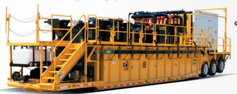
Ability to configure the reclaimer with or without a generator set mounted onboard
