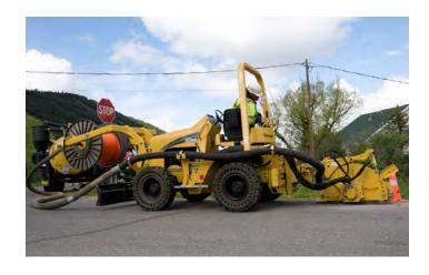
Then, there's the microtrencher MTR16 attachment. It has a maximum trench cutting depth of 16 inches (40.6 cm) and a width of 2.25 inches (5.7 cm). There are also two varieties of the MTR16 attachment to choose from:
